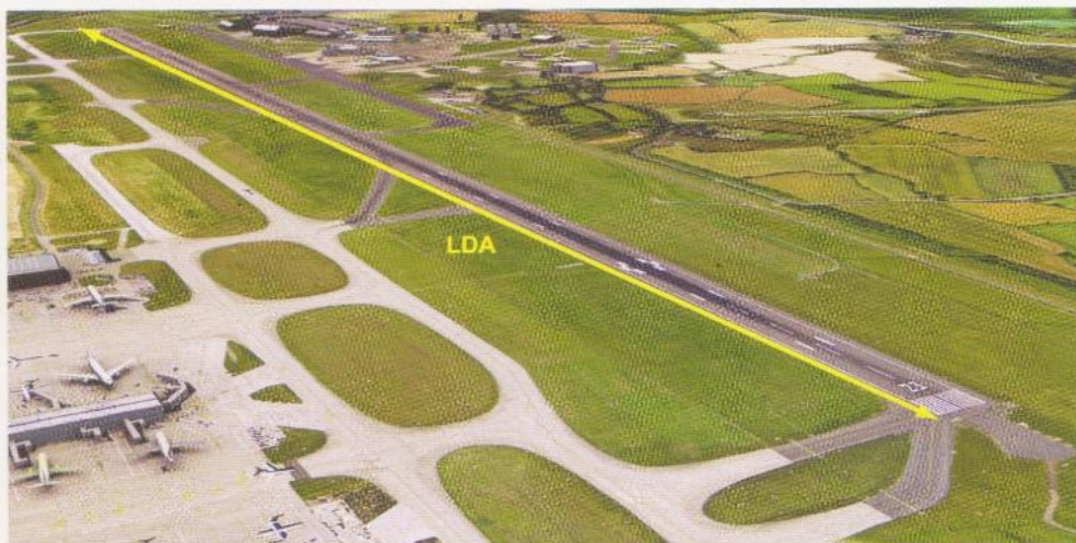
Figure 5.2 The Landing Distance Available (LDA) at an airfield is defined as being the length of runway suitable for landing.
