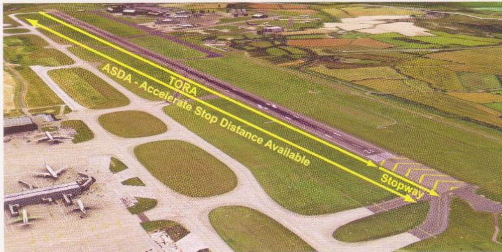
Figure 2.4 ASDA (Acceleration Stop Distance Available) = TORA + Stopway
