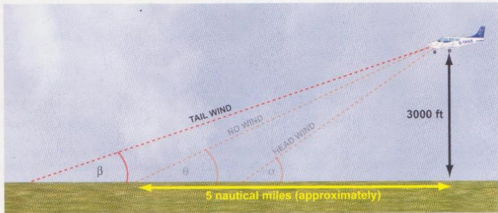
Figure 4.13 Headwind increases glide angle and decreases range. Tailwind decreases glide angle and increases range. With its 10:1 lift/drag ratio, clean, a Warrior will glide about 5 nm from a height of 3 000 feet.
