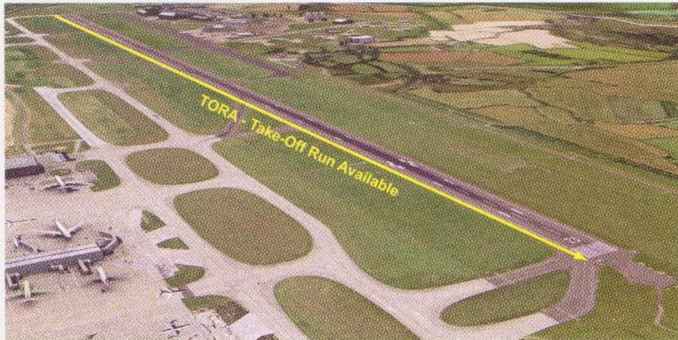
Figure 2.3 Take-Off Run Available - The length of runway suitable for the ground run of an aircraft on taking off.
