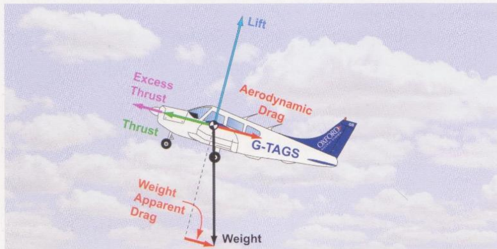
Figure 3.3 Forces in a steady climb showing excess thrust balancing weight apparent drag.
