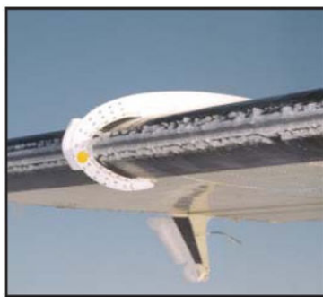
Mixed ice formation on wing leading edge
