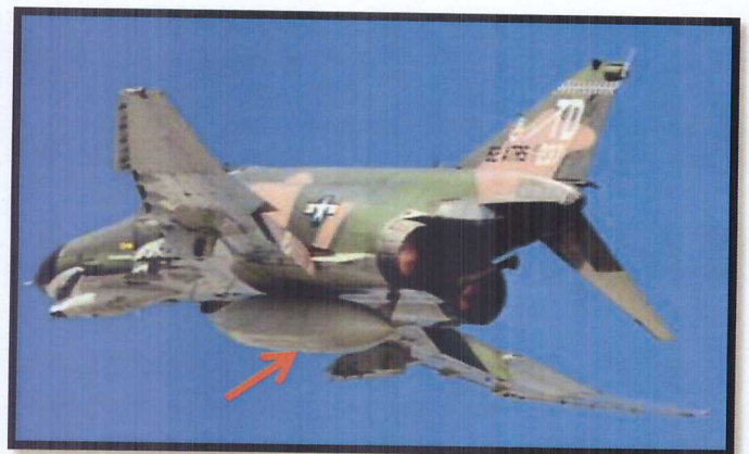
(External fuel tanks mounted under wings and fuselage of C-130 and F-4 aircraft)
