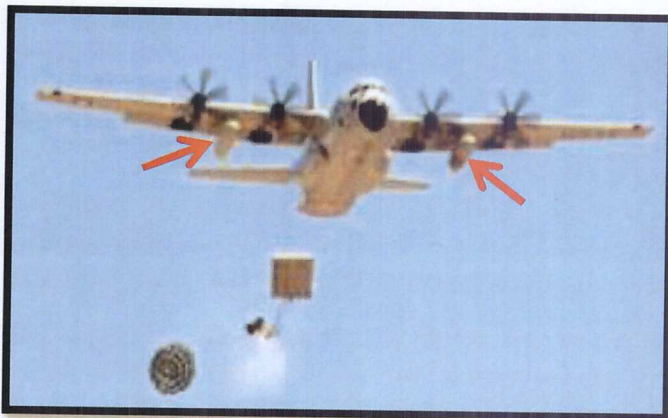
(External fuel tanks mounted under wings and fuselage of C-130 and F-4 aircraft)
